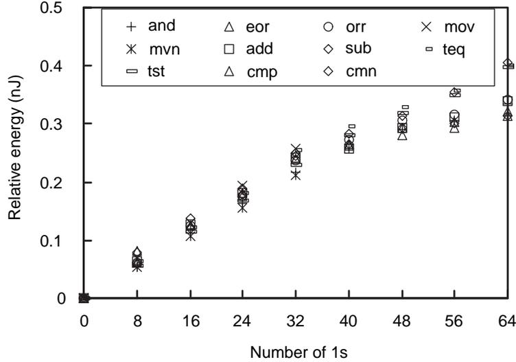
Figure 3: Energy consumption of the ARM7TDMI core by the operand values (EX stage)
