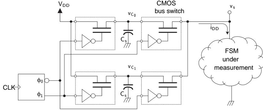
Figure 1: Measurement circuit using switched capacitors
