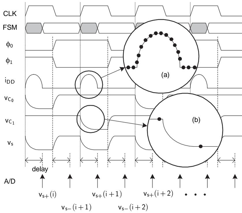
Figure 2: Waveforms of the clock-cycle-level energy consumption measurement system ((a): sample points for voltage measurement and (b): sample points for the proposed method)
