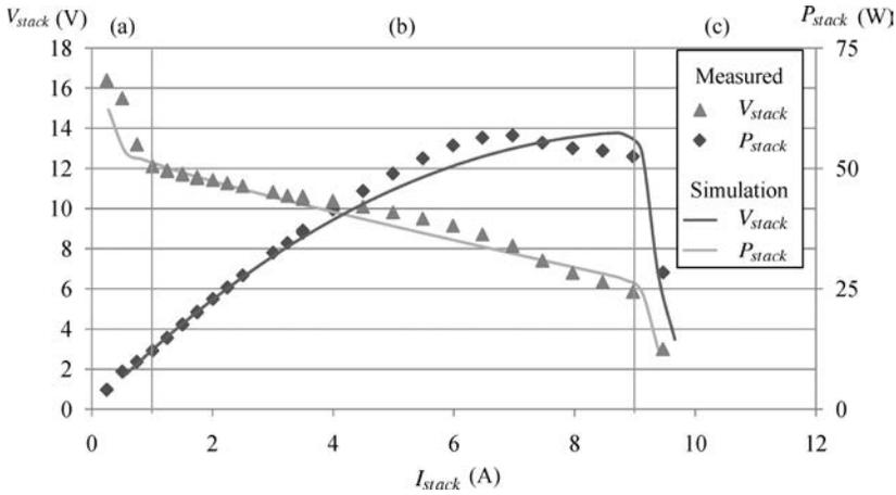
Fig. 6. DMFC stack voltage and current characteristic.
