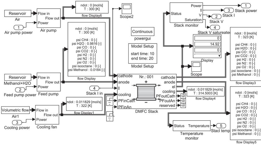
Fig. 13. DMFC system simulation setup using FCLib.
