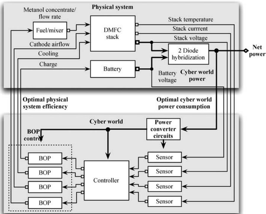
Fig. 1. Concept of the physical system and cyber world joint optimization of a portable active DMFC system.
