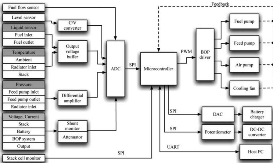
Fig. 8. Hardware platform architecture.
