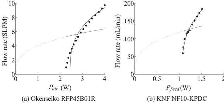
Fig. 3. Power consumption of BOP pumps.
