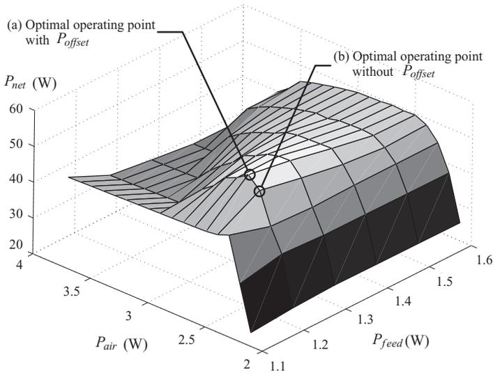
Fig. 14. Exploring the design space to achieve for the maximum net power of the DMFC system with an Okenseiko RFP45B01R blower.
