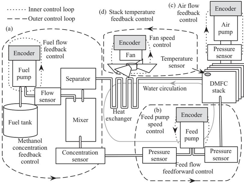
Fig. 11. Generic active DMFC BOP system architecture.
