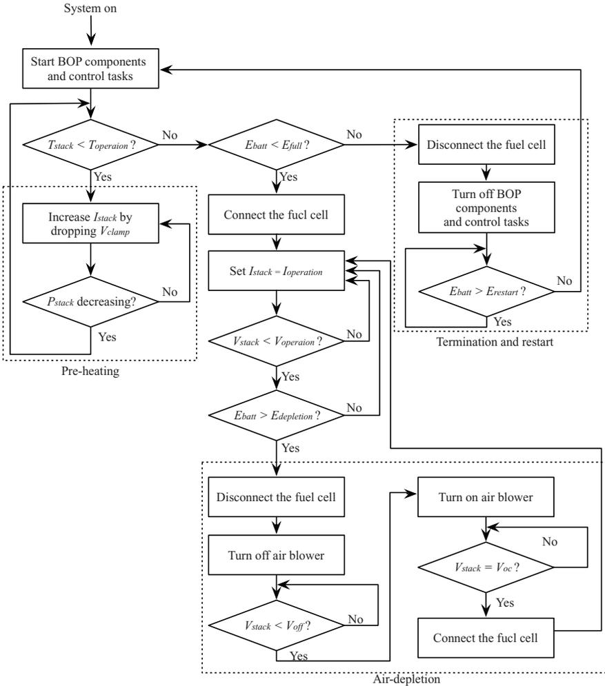
Fig. 12. Algorithm for system-level control.
