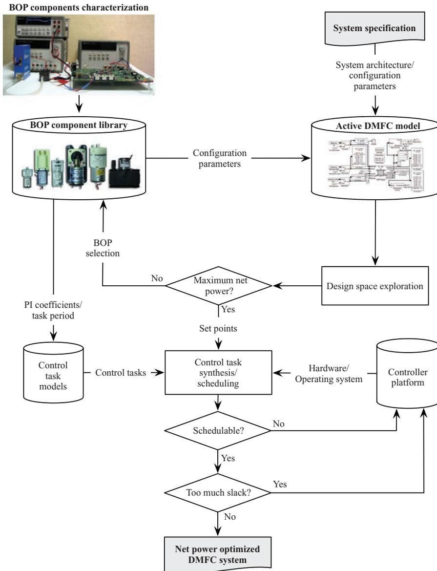
Fig. 2. Active DMFC system synthesis.
