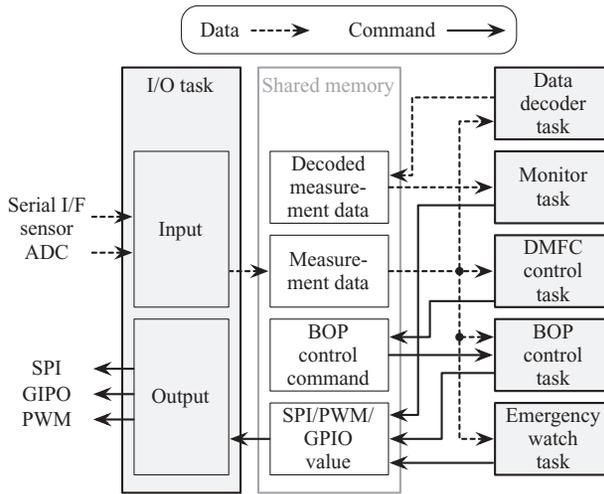
Fig. 10. Software block diagram and control/data flow.
