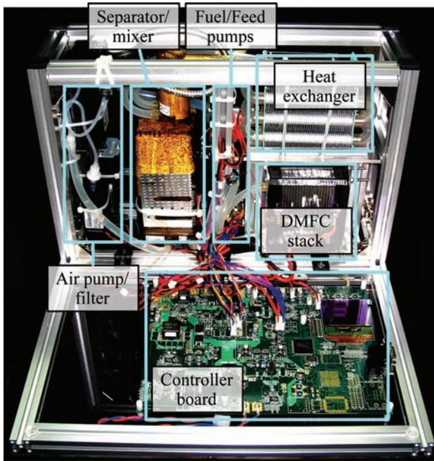
Fig. 16. Implemented DMFC system prototype.
