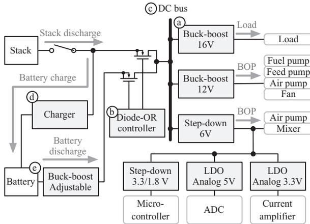
Fig. 9. DC power distribution path and power-up sequence. Circled numbers denote the order in which components are enabled.
