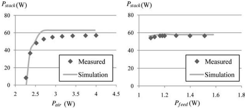
Fig. 7. DMFC stack power with different BOP power.
