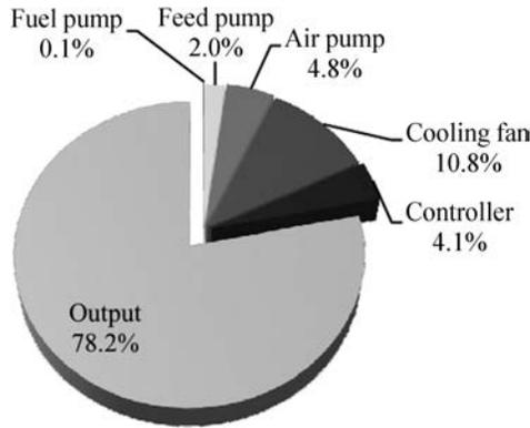
Fig. 17. Destination of the power generated by the stack in our prototype DMFC system.
