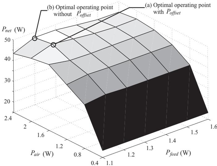
Fig. 15. Design space exploration for the maximum net power of the DMFC system with Okenseiko P09A03R.
