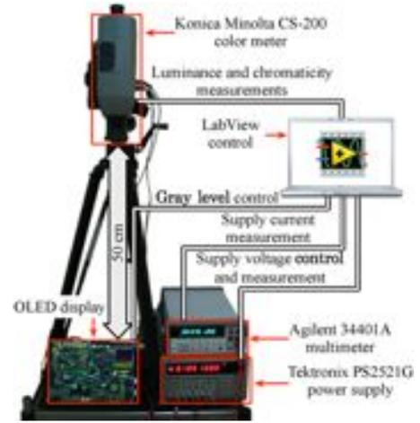
Fig. 6. Experimental setup for the OLED display panel characterization.
